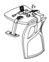
Assemble the back to the seat, tighten the bolt firmly.
