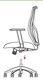
Insert cylinder into the housing of the mechanism attached to the seat.
