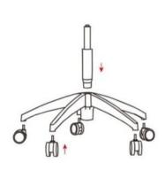
Place the cylinder and caster firmly into the base.
